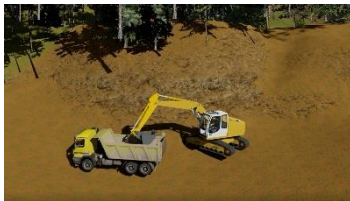
Gambar 5. Ilustrasi Galian Spillway
