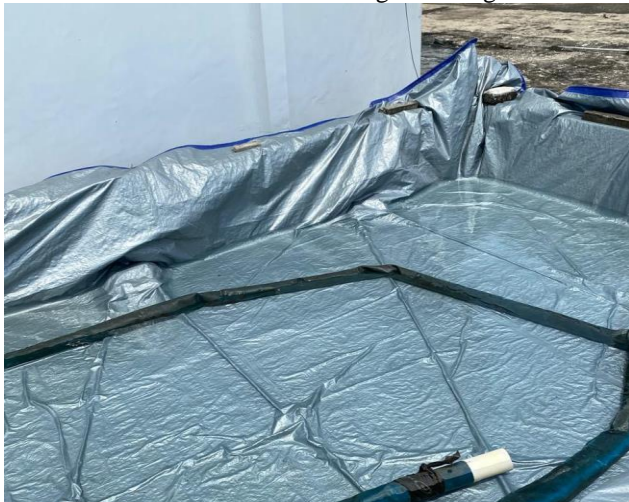
Gambar 6 Kolam Air Static Loading Test
