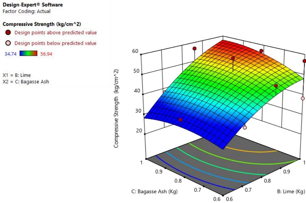
**Figure 5.** Surface response of the effect of lime and SCBA on compressive strength
