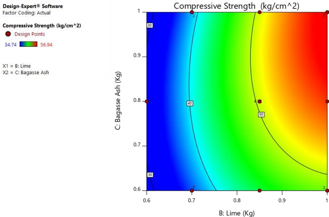
**Figure 6.** Contour plot of the effect of lime and SCBA on compressive strength
