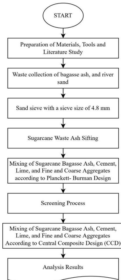
**Figure 1.** Research procedure for making concrete bricks from sugarcane bagasse
